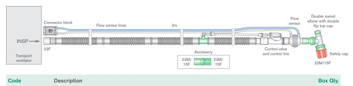
2072000 22mm Flextube™ transport breathing system, for use with Oxylog® 3000, 3000 plus and 2000 plus, 2m 10
